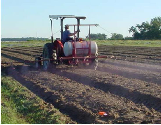
Figure 1. Boom set-up for extended flat-fan nozzles and location of card holders.
