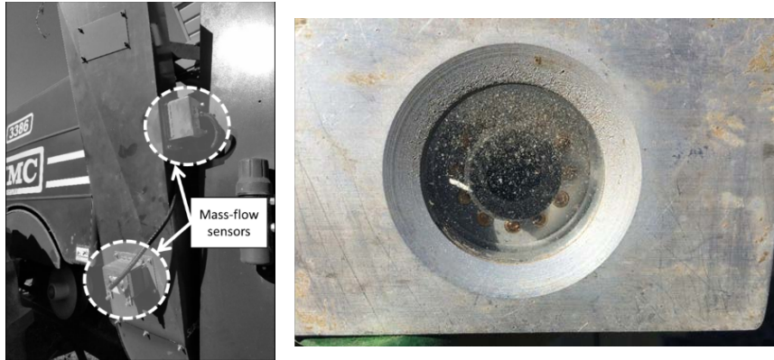
Figure 1. Mounting location of the two mass flow sensors on the duct of a KMC 3386 combine (left) and lens of the sensor located at the lower position showing abrasion and pitting from the pebbles and other foreign material (right).
