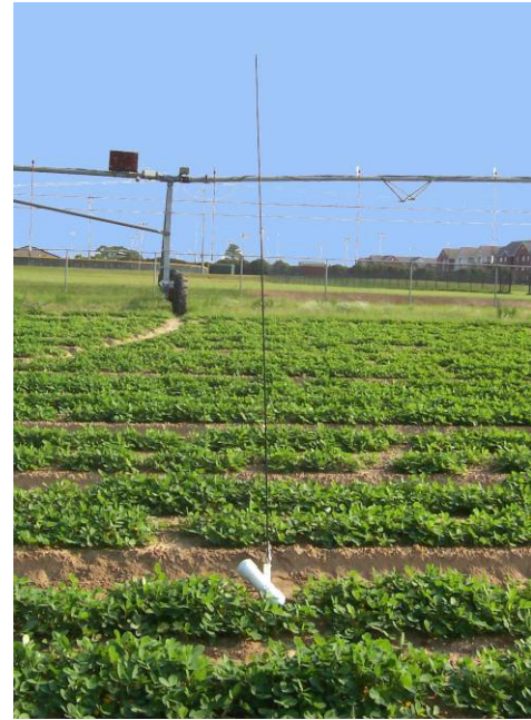
Figure 1. To overcome the range issue, the original mote antennas were enclosed in an 8 foot, 0.25 inch diameter hollow, flexible, fiberglass rod. The rods were mounted to a PVC pipe used as a supporting stake with a spring used for conventional CB antennas. The pipe also supported the PVC enclosure housing the node circuitry including the Mica2 motes.
