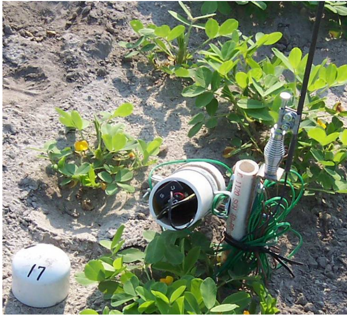
Figure 1. To overcome the range issue, the original mote antennas were enclosed in an 8 foot, 0.25 inch diameter hollow, flexible, fiberglass rod. The rods were mounted to a PVC pipe used as a supporting stake with a spring used for conventional CB antennas. The pipe also supported the PVC enclosure housing the node circuitry including the Mica2 motes.
