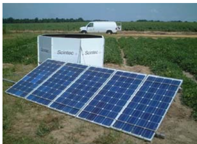
Figure 3. Solar-powered sodar setup for wind speed and direction measurements.
